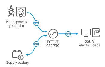
ECTIVE CSI PRO inverters convert direct current from a supply battery into high-quality alternating current with a pure sine wave. This means that sophisticated 230 V devices can be operated anywhere and anytime: exactly like with a power outlet at home.
