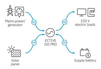
ECTIVE SSI PRO inverters convert direct current from a supply battery into high-quality alternating current with a pure sine wave. This means that sophisticated 230 V devices can be operated anywhere and anytime: exactly like with a power outlet at home.
