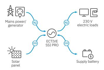
a supply battery into high-quality alternating current with a pure sine wave. This means that sophisticated 230 V devices can be operated anywhere and anytime: exactly like with a power outlet at home.
